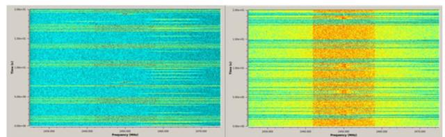
Fig. 1 LTE-U transmissions for duty cycle 10% and 90% respectively
