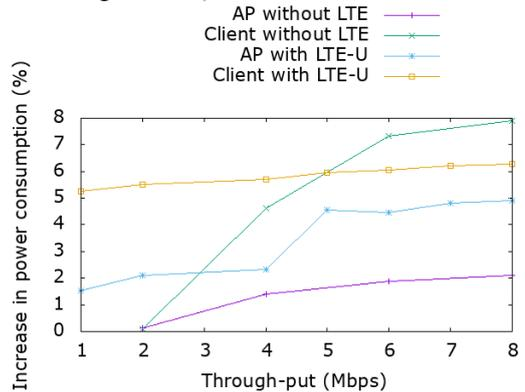
Fig. 15 Comparison between the scenarios with or without LTE-U interference
