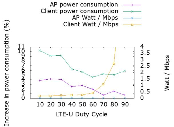
Fig. 14 Measure of WiFi node power consumption for various traffic loads with LTE-U interference
