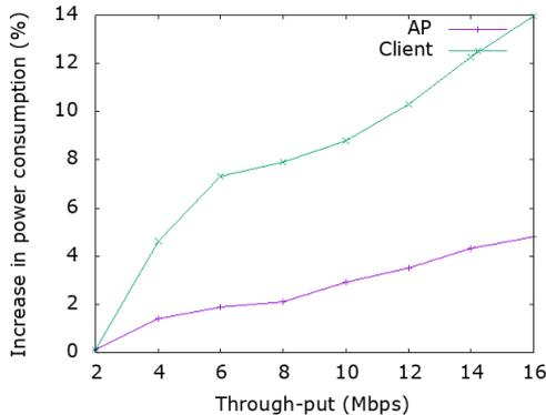
Fig. 13 Measure of WiFi node power consumption for various traffic loads
