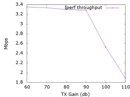
Fig. 6 Tx Gain of LTE radio impact on WiFi performance
