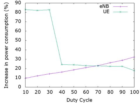
Fig. 10 LTE's UE and eNB power consumption when Duty Cycle concept is implemented
