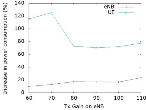
Fig. 12 Tx Gain of LTE eNB impact on UE and eNB power consumption
