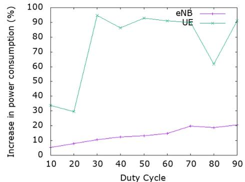
Fig. 11 LTE's UE and eNB power consumption with a fully saturated WiFi link
