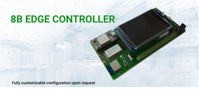
The 8B Edge Controller consists of a single core 32-bit ARM® Cortex®-M4, a dual core 32-bit Xtensa®, 1-Mbyte Flash memory and 192-KByte RAM. The platform is programmable via USB, it has a MicroSD storage slot for up to 64GB cards and can transmit data via Bluetooth and WiFi.
