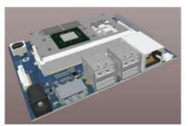
The 8B Edge Controller consists of a single core 32-bit ARM® Cortex®-M4, a dual core 32-bit Xtensa®, 1-Mbyte Flash memory and 192-KByte RAM. The platform is programmable via a USB connection, it has a MicroSD storage slot for up to 64GB cards, and it can transmit data via Bluetooth and WiFi.
